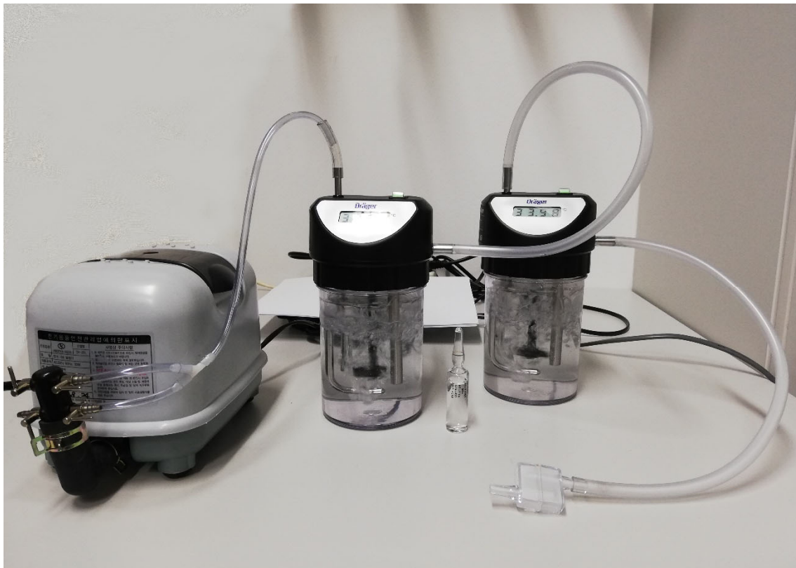
Figure 4: Experimental setup for the conduction of the accuracy study for breath alcohol measuring devices. The membrane pump is visible on the left side, the two simulators operated in series are located to the right of it. The test gas is passed through the hose in the foreground at the end of which there is a droplet trap and presented to the measuring devices. Between the simulators an ampoule with an alcohol reference solution is shown, as is used to prepare the standards.
